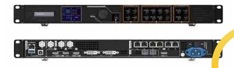
The VX600 is NovaStar's new all-in-one controller that integrates video processing and video control into one box.
