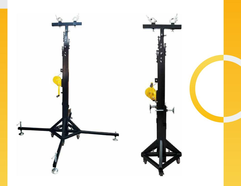
Heavy hand tower lift, Materials for iron, highest can rise to 6 M height, low of 2.06 M, bottom spread: 2.1 x 2.1 M, pack up the bottom,  $46 \times 46$  CM, the four leg, Bar length: 50 CM,. load weight: 250 KG
